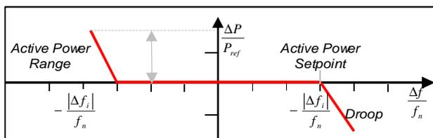
Figure 4: Variation of the power output of generating systems
