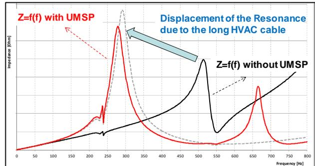
Figure 2: Impact to the Impedance-Frequency-Curve
