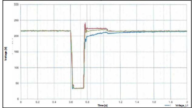
Figure 8: Real FRT measure at LV side
