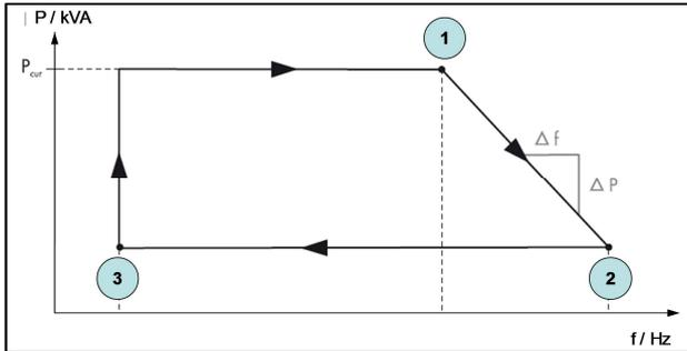
Figure 6: Principle for the active power regulation
